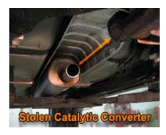
Since 1975, all vehicles produced in the United States must have a catalytic converter as part of the exhaust system. The catalytic converter is an emissions-control device that contains precious metals that act as catalysts. When hot exhaust enters the converter, a chemical reaction occurs that renders toxic gases, such as carbon monoxide and hydrocarbons, into less harmful emissions.
